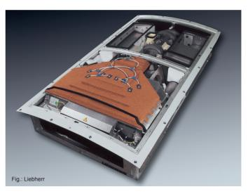
ICE3 high-speed train Roof-mounted air handling unit with RF22P housing fan
